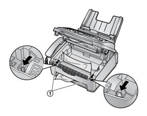
**5** Remove the jammed paper (①) from the fuser unit by pulling it upwards carefully, then install the drum and toner unit.
